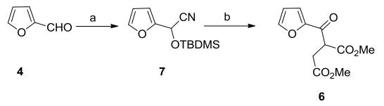
Scheme 1: Synthesis of furan diester 6. Conditions: a) TBSCl, KCN, ZnI<sub>2</sub>, MeCN, 12 h, rt (96%); b) (i) LDA, dimethylmaleate, THF, 1 h, -78 °C; (ii) TBAF, HAc, THF, rt, 4h (61%).
